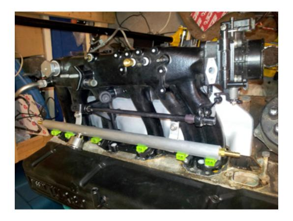
Ported Datsun 280ZXT turbo manifold. This manifold had been heavily modified to allow for much better breathing. The stock intake runners are almost half the volume of the stock intake valves. This manifold removes the #1 choking point of the L series turbo engines.
