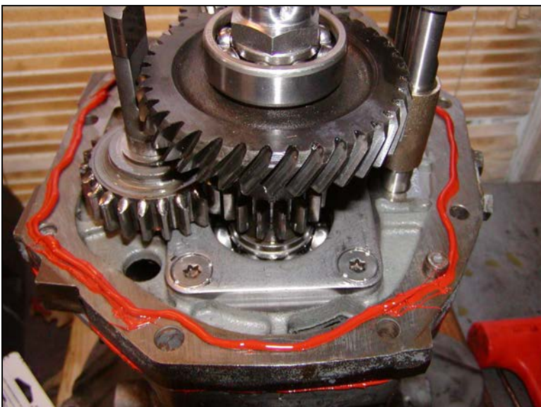
Photo 55—Sealant applied to adapter plate, following around the outsides of the bolt holes.
