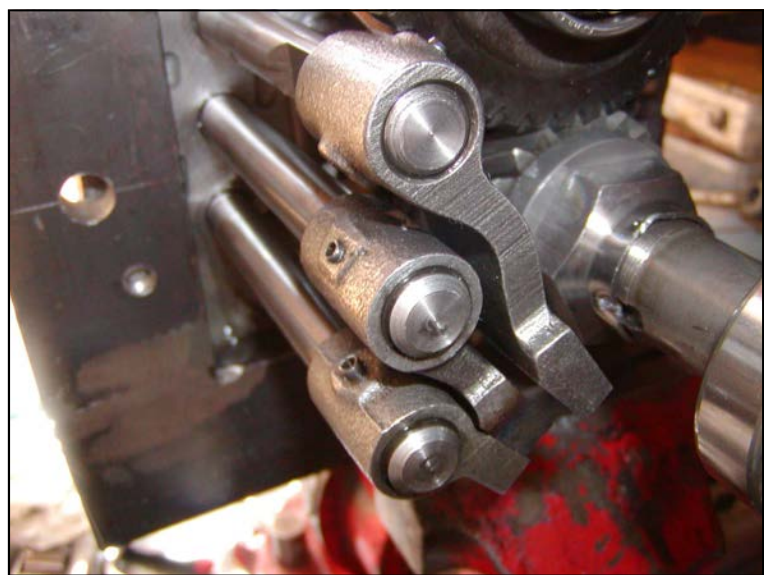
Photo 51—Striking lever gate of the shift fork rod should be facing the 4 o'clock position, as shown here.
