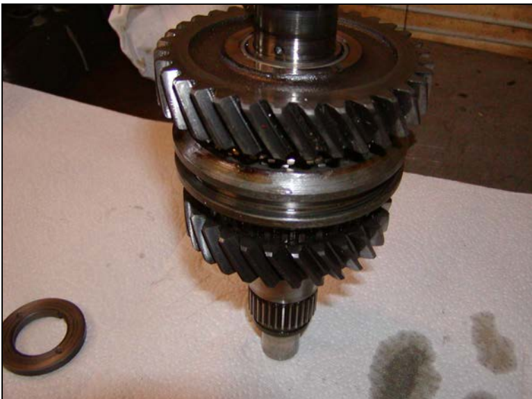
Photo 38—Assembly of the 1st/2nd gear synchronizer hub assembly.
