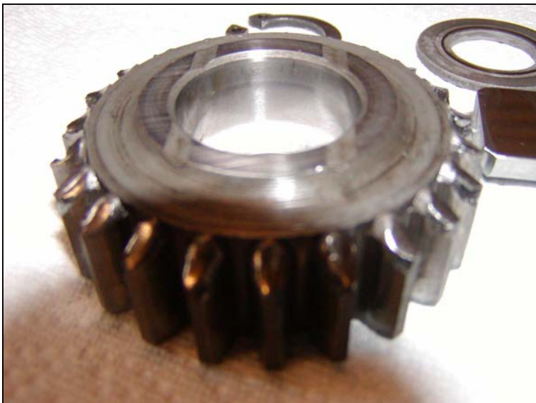
Photo 19—Inspection of the reverse idler gear shows extreme wear on the teeth. Replacement is necessary.
