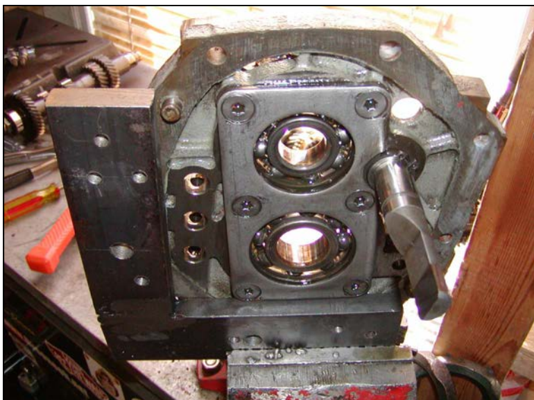
Photo 16—Transmission adapter plate shown mostly disassembled. Remove the bearing retainer plate next.
