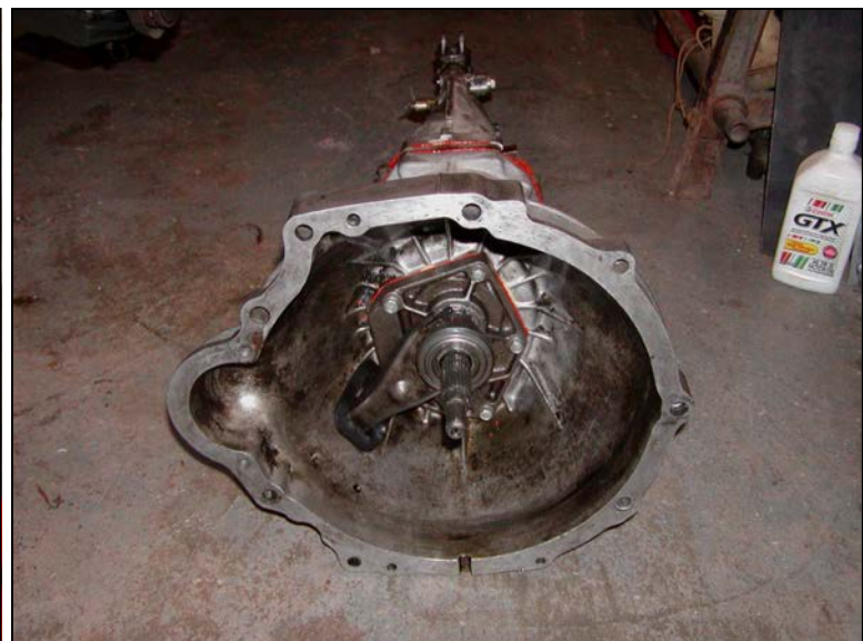
Photo 60—Finished, rebuilt transmission ready to install.
