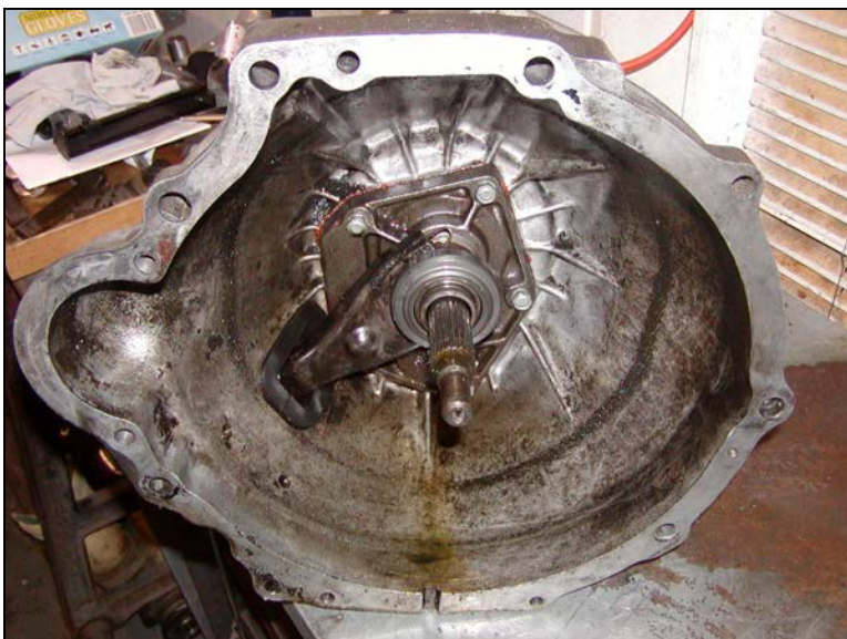
Photo 2—Bellhousing of the FS5W71, including the input shaft, throw out bearing, and clutch fork.
