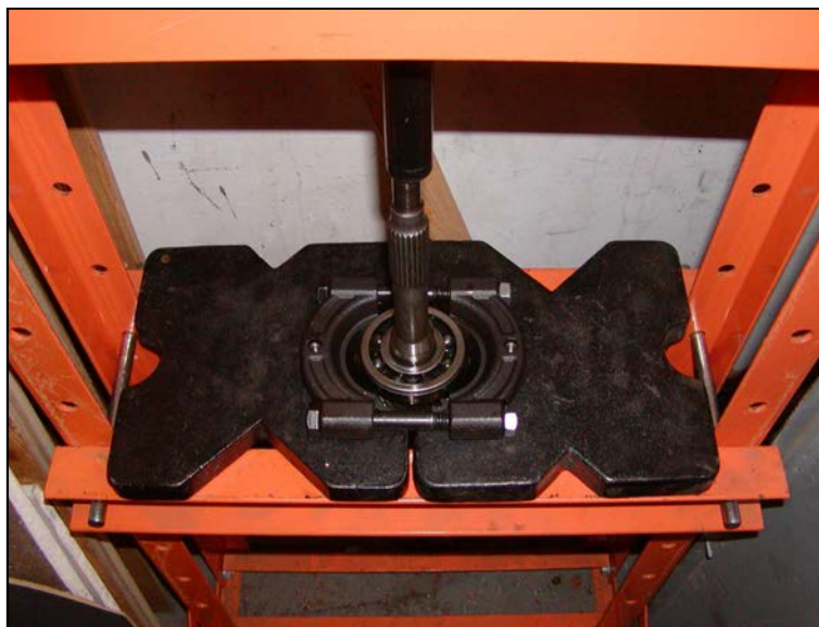
Photo 17—Positioning shown for pressing off the input shaft bearing.
