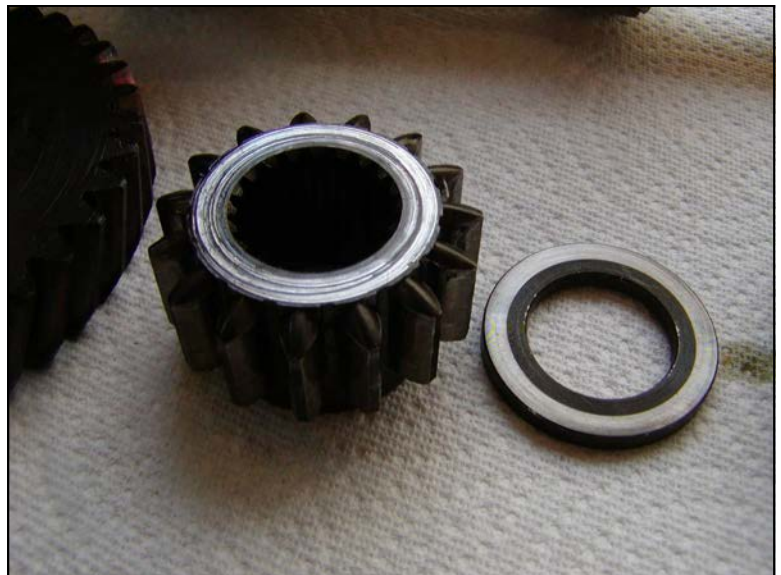
Photo 30—Countershaft drive gear face shows light scoring.
