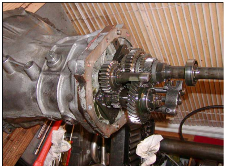
Photo 4—Tailshaft case section removed, exposing some of the internal transmission gears.
