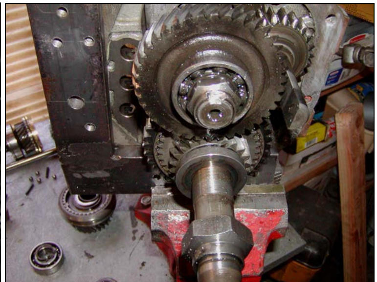
Photo 14—Countershaft nut staking removed, here using a die grinder. Ensure no damage to the shaft or
