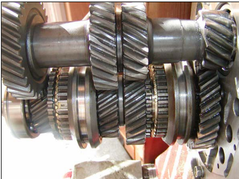
Photo 47—Gears shown here are double-engaged to enable tightening of the mainshaft nut.
