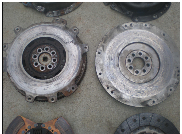
Photo 3—6-speed flywheel shown on the left, compared to an S13 flywheel shown on the right. Mounting pattern for the pressure plate is the same, but pilot bushing is housed in the 6-speed flywheel.
