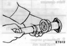
Fig. ET-7 Testing Radiator Cap
